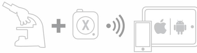
The **Moticam X**, like all our Moticam solutions, is an “All-In-One-Box” product. What makes the Moticam X a cut above the rest is that it is a high resolution streaming **WiFi camera**. By creating its own wireless network, simply logon with your Android or iOS tablet and **view, capture, edit live images** from your microscope with our **free App MotiConnect**.
